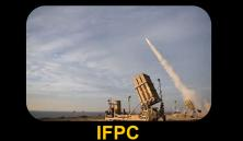
Indirect Fire Protection Capability System is a mobile, ground-based weapon system designed to defeat cruise missiles (CM), unmanned aircraft systems (UAS), and rocket, artillery, and mortars (RAM).
