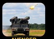
Avenger's lethality and mobility protects maneuver forces and critical assets with a rapid fire missile system that acquires, tracks, and engages low-altitude threats. The Avenger is capable of shooting on the move to destroy aerial threats with Stinger missiles and the M3P .50-caliber machine gun.
